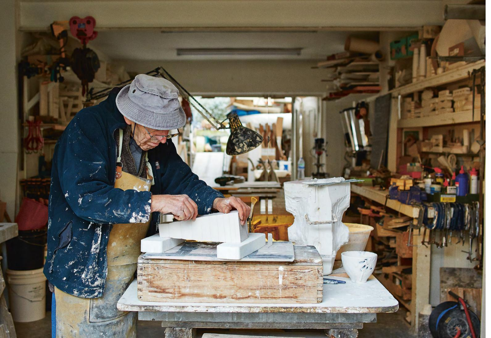
Making plaster protoype moulds for works in progress in his workshop
